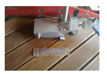
Customer: Wallbarn Ltd Test Number: FS10174 Operator: Glenn MacLaughlan Date of Test: 20th April 2016 On Site: Samples sent to office Pendulum Calibration Number: CN302 Pendulum serial number: SK1698 Slider Type :Fours 96 Contaminate Description: Water Reference: IPE - Timber Tiles
