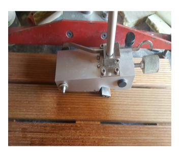
Customer: Wallbarn Ltd Test Number: FS10174 Operator: Glenn MacLaughlan Date of Test: 20th April 2016 On Site: Samples sent to office Pendulum Calibration Number: CN302 Pendulum serial number: SK1698 Slider Type :Fours 96 Contaminate Description: Water Reference: Cumaru - Timber Tiles
