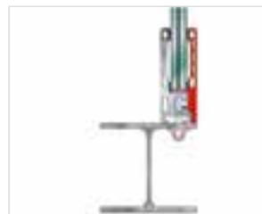
Installation on steel, direct installation from above
