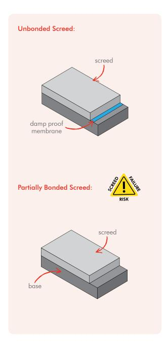
Partially bonded screeds are not recommended by Flowcrete for industrial or commercial purposes as the finish is prone to cracking. In this form of application the screed is laid directly onto unprepared concrete and it cannot be guaranteed to achieve a bond across 100% of the area. You can tell where it hasn't bonded by tapping the dried screed and listening for a hollow sound, meaning it has not bonded.
