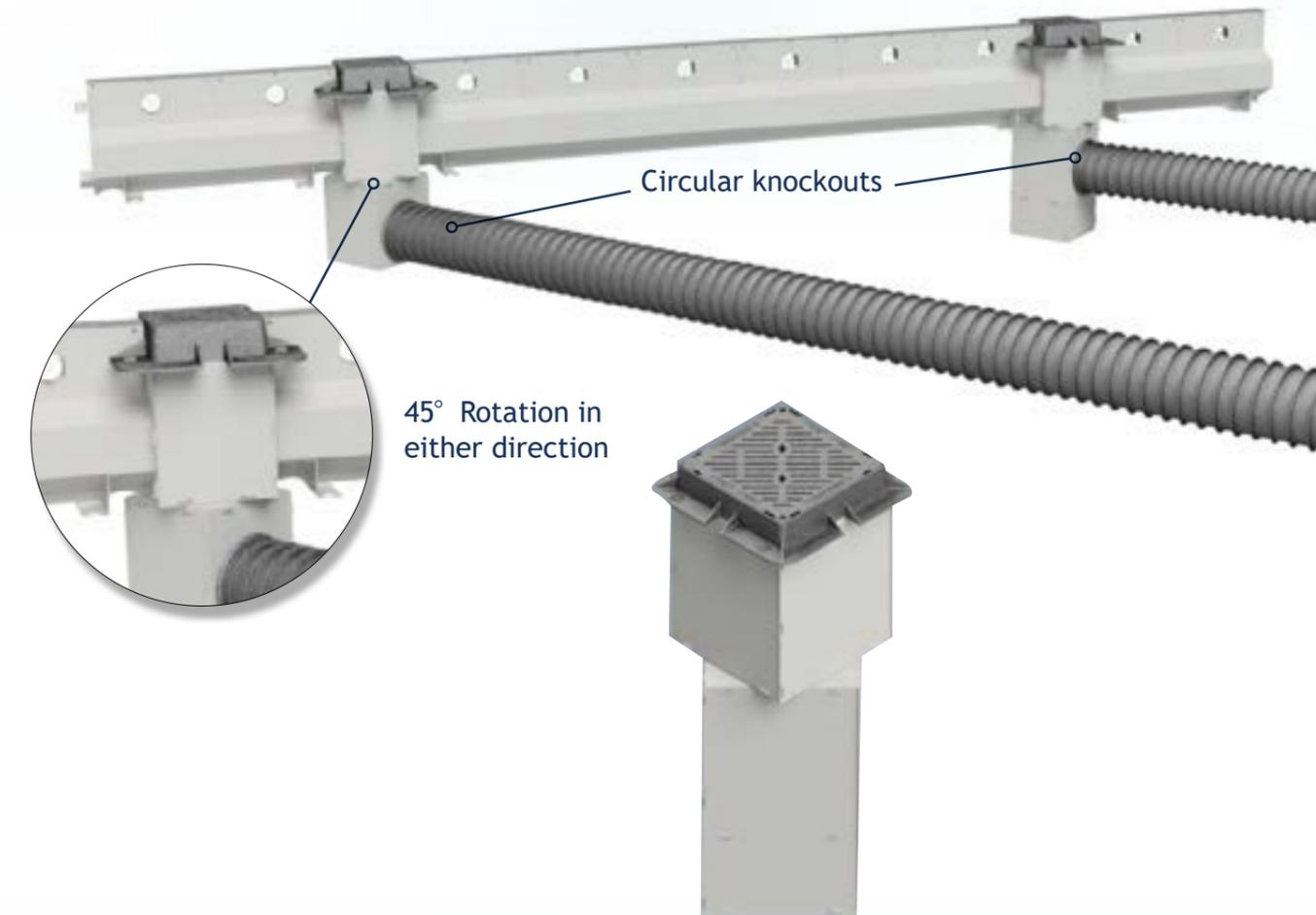
The Gatic Roto Modular range features a pivoting function that allows the lower section to rotate 45° in either direction.
