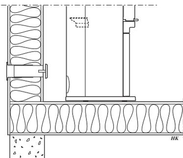
Indirect air supply through the external wall.
