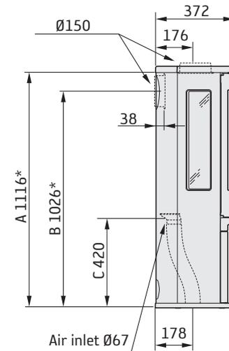
The minimum distance in front of the stove opening to combustible parts of the building or interior decoration must be at least 1 m.
