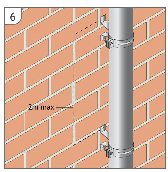
Downpipes should be installed using at least 2/no pipe clips per length. Mark out the clips locations and level with a sprit level or plumb line. Open the tightening screw to allow the pipe to be inserted, close the clip and re-tighten, making sure not to over tighten and damage the downpipe.
