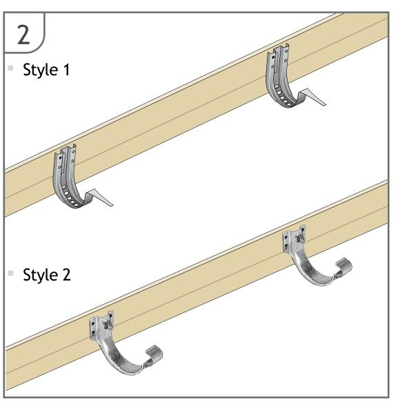
Use a string line to set out your fascia brackets along the gutter run allowing for a fall of 1:600 to 1:350 (max).
