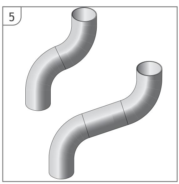
Offsets are achieved using 2/no 70° bends, with larger offsets being made by inserting a pipe length between the two bends.
