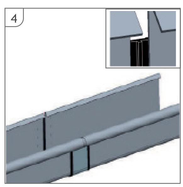
Attach the sealing strip over both ends of the gutters, starting at the 'bead/roll' at the front edge. Keep a slight tension on the strip to stretch round to the back while also smoothing/pressing down for a good bond.
