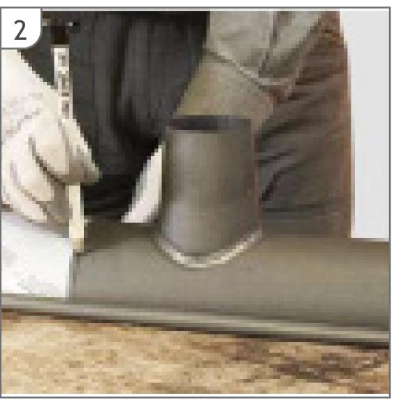
Cut the running outlet to the required length, starting from the rolled front edge.
