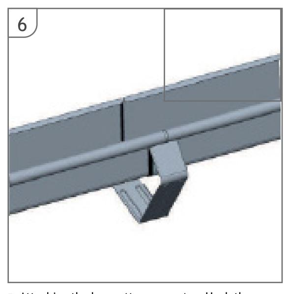
Attaching the box gutter connector: Hook the connector onto the bead at the front first, then pressing onto the adhesive surfaces of the seal throughout, wrap it around the gutter lengths over the join to the back.
