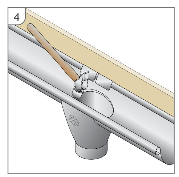
Tap the inner rough edges of the hole that was cut in the gutter, down into the outlet, to ensure a smooth flow of water.
