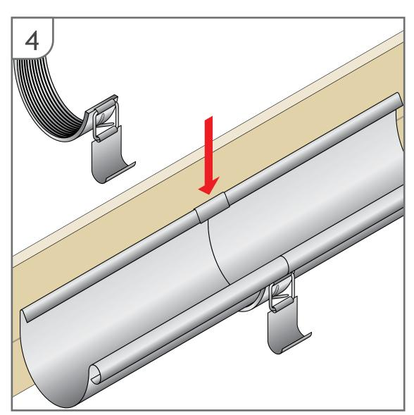
An EDPM rubber sealed union connector is used to connect the gutter lengths and angles together.
