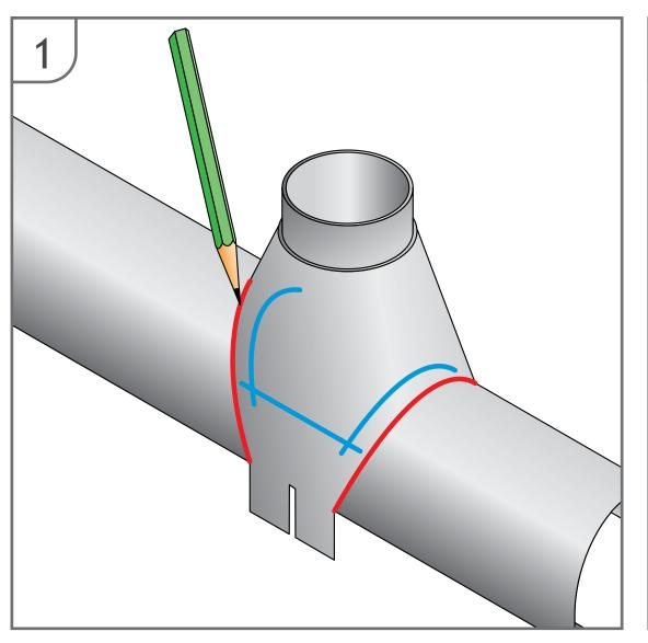
When installing a 'wrap around outlet' mark the desired location of the outlet by drawing a line either side of the outlet along its edge. Draw a further line 20mm inside of the outer lines and join these inner lines together in an oval pattern. This becomes the marking for the cut out hole.
