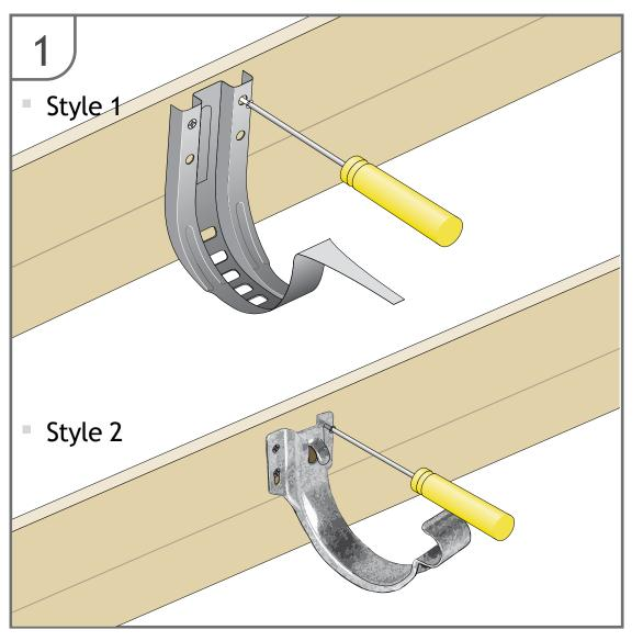
Generally position the fascia brackets at 915mm centres, using at least 3 brackets per gutter length. Use 2 screws on both the left and right fixing options and 1/no underneath the gutter securing tab.
