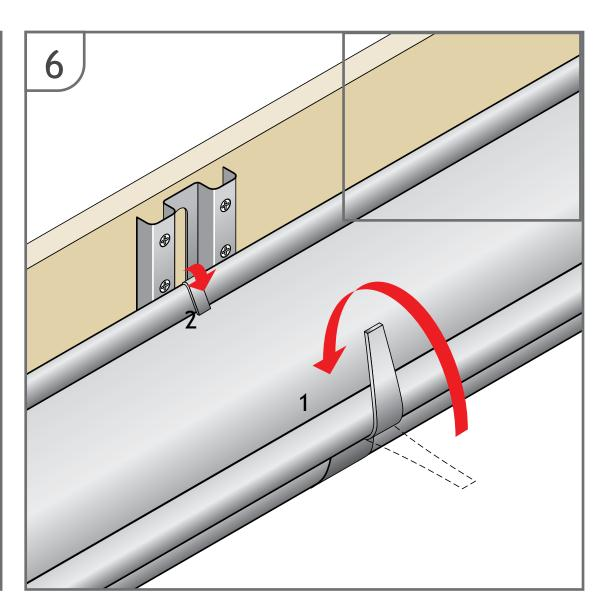
Locate the gutter into the fascia bracket and seat level, then fold the front tab of the fascia bracket around the front roll and into the gutter. Fold the rear tab of the fascia bracket down and over the rear edge of the gutter.
