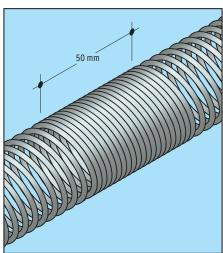
The connection between two sections of Spiral drain is done by entwining together for a 50mm section.
