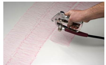
Correct application of adhesive
