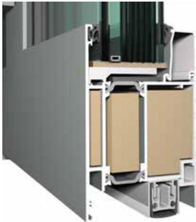
The CS 77-FP EI30 and EI60 is developed based on the existing CS 77 profiles and accessories for windows and doors and extensively tested in an optimized European test and approval program. The fireproofing time span is achieved by inducing a special cooling material into the profile chambers and by using self-adhesive and water-resistant swelling gaskets. These gaskets do not need to be sealed, reducing fabrication time of the profiles and saving costs.
