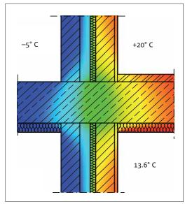
Balcony connection without thermal break. Insulation under balcony and ceiling.
