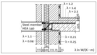
Connection of steel member HEA 140 with Schöck Isokorb® type KS14 and a composite thermal insulation system
