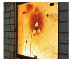
Test: Large fire test after gun shots
