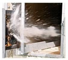
Test: Gun shots after small fire test
