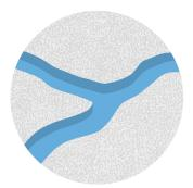
Conventional concrete contains capillaries, making it naturally porous
