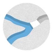
Hydrophobic admixture forms barrier inside capillaries during the hydration process.
