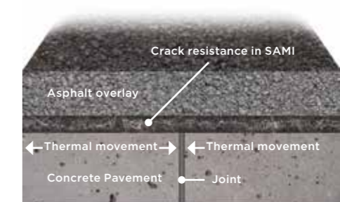
ASPHALT OVERLAY WITH ULTILAYER SAMI
